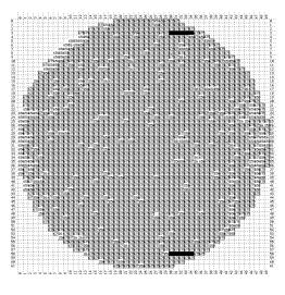
Figure 4 Map of failures from programmed wafer after forming gas anneal. Failures appear dark.
