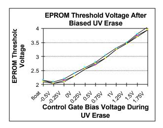
Figure 3 EPROM threshold voltage after biased UV erase
